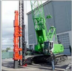
Hydraulic add-on vibrators or excavator attachments are the ideal tool to convert standard excavators into powerful piling machines for sheet piles, beams and pipes of shorter lengths.
