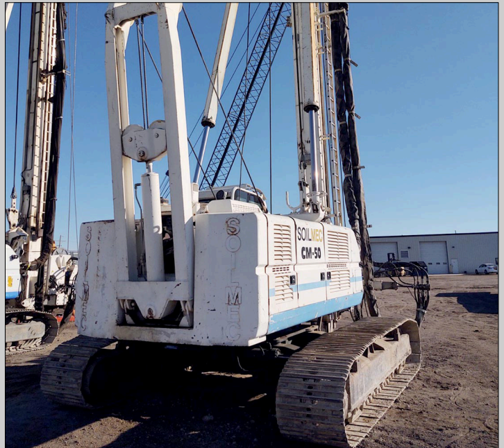
Soilmec CM 50 CFA drilling depth 25 m with 6 m extension Torque 100 kN, weight 40 ton, Jean Lutz computer YOM 2006, hours ~9000, very good condition
