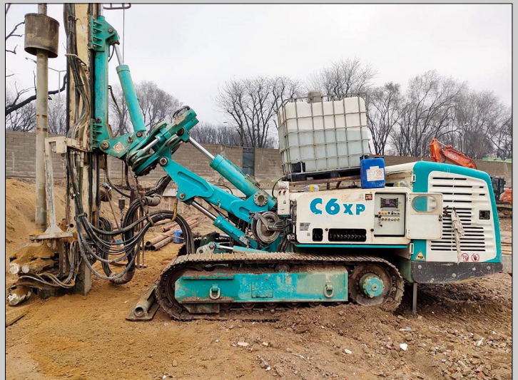
Casagrande C6 XP Drill head T20, clamps \varnothing 360 mm Foam pump, lubricator, radio control YOM 2014, hours ~9250, serviced & painted
