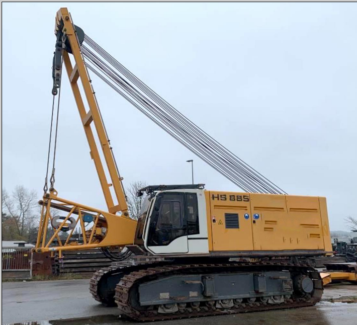
Liebherr HS885 HD Litronic Winches 2 x 30 ton free-fall Engine 670 kW, boom length ~30,50 m YOM 2015, hours ~7990, very good condition
