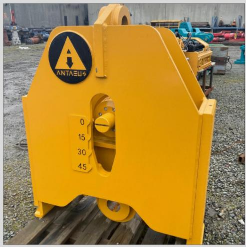
The Antaeus NO SHOCK is designed to protect telescopic booms on all cranes, including truck cranes
