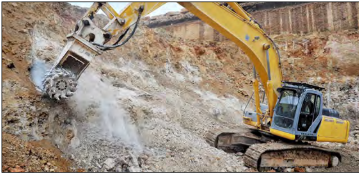
ADD-ON DRUM CUTTERS For cutting rock & concrete
