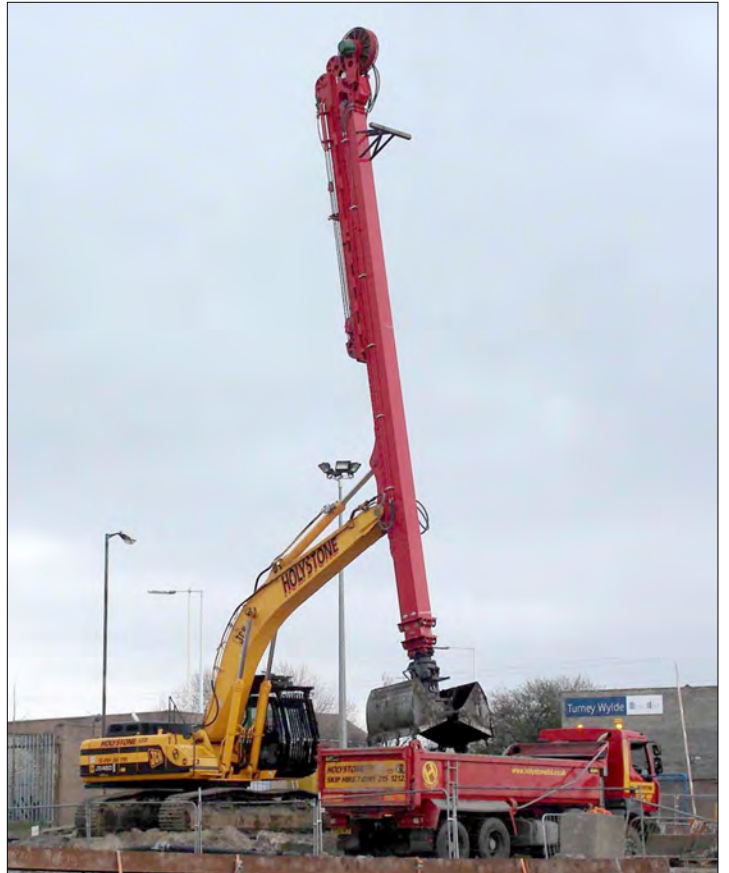
ADD-ON TELEDIPPER Extending the reach of excavators up to 34 m depth
