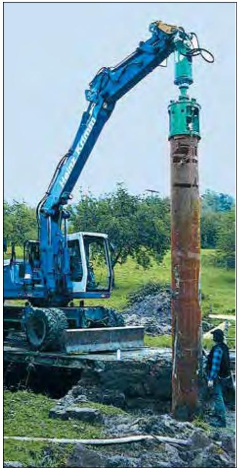
You may be surprised what your excavator can do with dedicated, top quality attachments, mounted to the boom stick and connected to the hydraulic circuit of the base machine:
